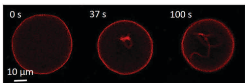
Fig. 5 Time lapse of a DOPC vesicle with 2 mol% TR-DHPE developing inward nanotubes as a result of long exposure to laser during confocal imaging. The second and third cross sections are non-equatorial to better show the formed nanotubes.
